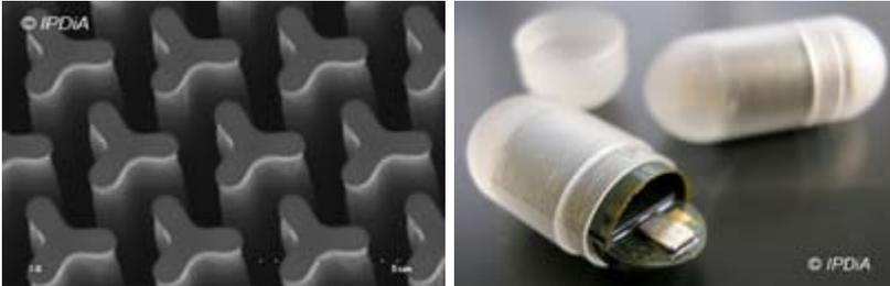
*Picture right: Prototype of medical pills integrating temperature sensor and RF transceiver
